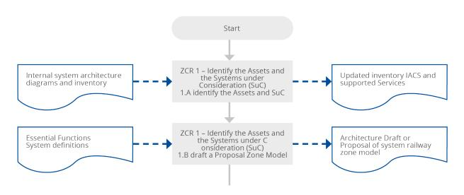
Figure 3 illustrates the steps to be applied to perform the initial risk assessment as a second step and to derive a security architecture in 'zones and conduits'.
