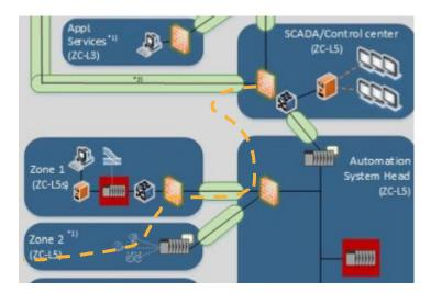
7) Place means for monitoring management systems (technical domain controller, network management, NAC, PKI, Syslog & SIEM, etc.) in every organisational SuC to support the 'de-centralised approach' and the 'modular entity subsystem approach'.
