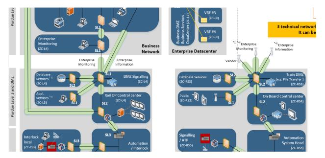
Depending on the location in the company model, this results in a strengthening of the encryption and security features of the security gateways between each zone and conduit.
