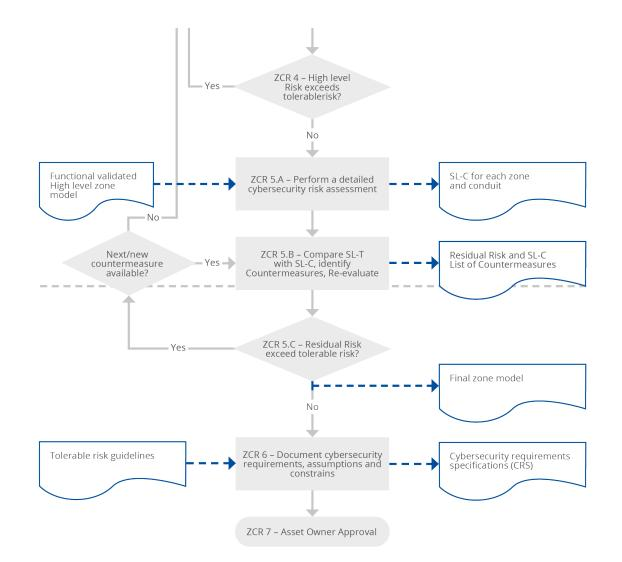
The final zone model depends on existing systems and zones, the result of the threat risk assessment and the target architecture of each railway operator. Security parameters such as security levels (SL), zone criticality (ZC) or protection profiles are discussed in separate chapters and are built upon of this generic base.
